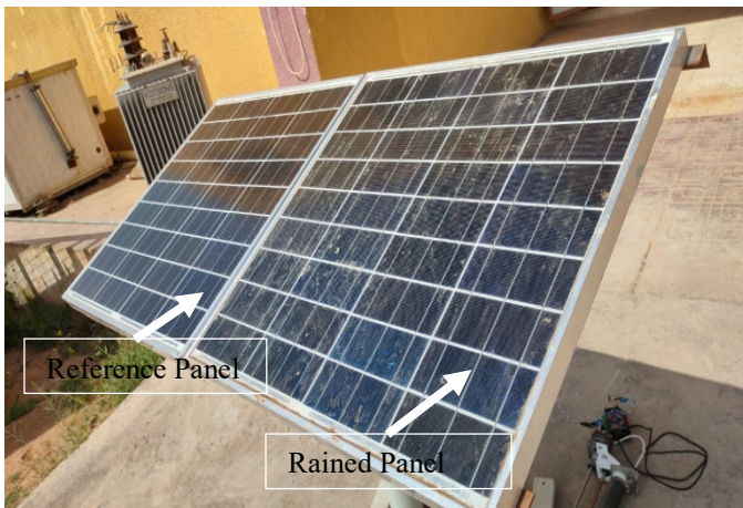
Fig. 5. The reference panel is on the left and the rained panel is on the right.
