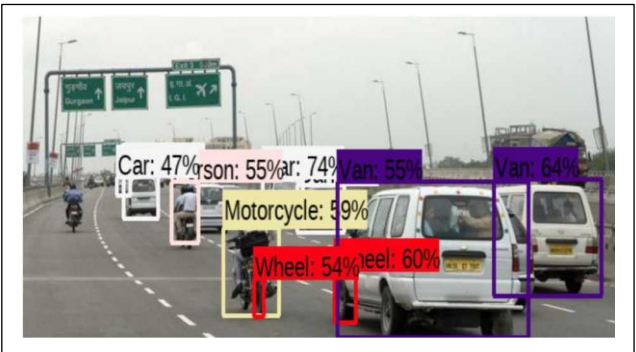
Figure (3-b): Moving vehicles image as detected by R-CNN
