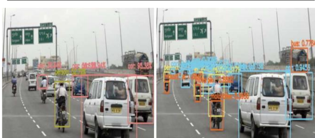
Figure (3-a): Moving vehicles image as detected by YOLO (left) and SSD (right)
