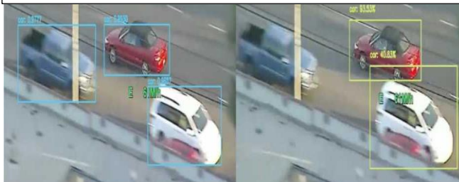
Figure (4): Video object detection for accident YOLO (left) and SSD (right)
