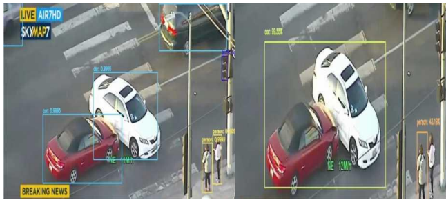
Figure (4): Video object detection for accident YOLO (left) and SSD (right)
