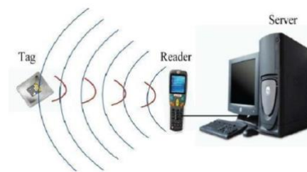
Figure 1: Relationship between RFID Tag, Reader, and Host Computer (Diyari Qadir Mohammed, 2021)
