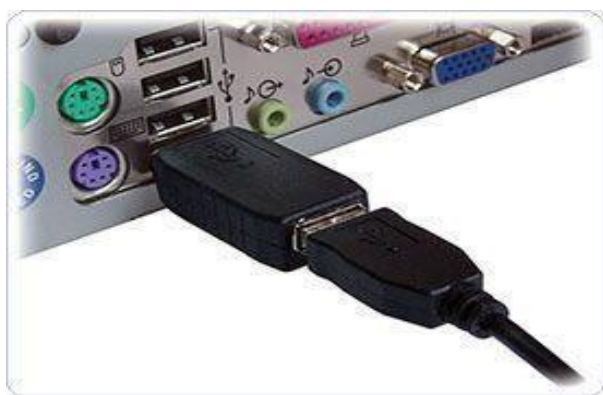
Figure 1. A Hardware keylogger on USB port
