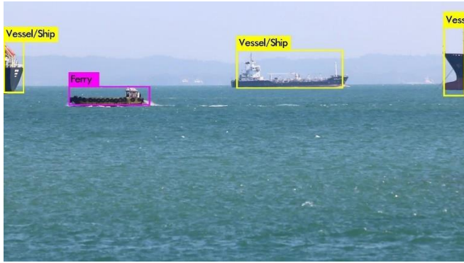
Figure 4: detection result from video 1, the framework detected 2 types of ships.
