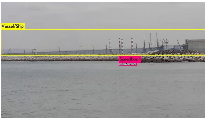
Figure 6: detection results from video 3, where a small speedboat is detected, but the environment around it is classified incorrectly.
